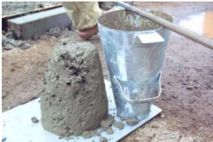
Fig 14. Photograph of slump test of glass cullet concrete
