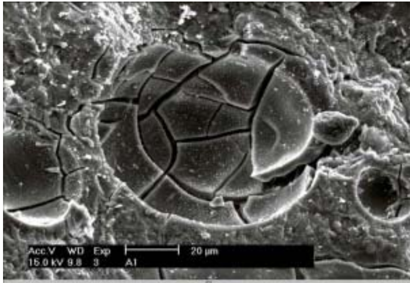
Fig 8. Probable gel formation in ASR test sample
